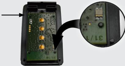
5) Replace the electronic card with the new battery in the box. The fixing plates and the dimensions of the electronic card mean that it must be correctly reassembled.
