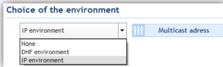
**IP Environment** enables the master clock to control devices through Ethernet network.
