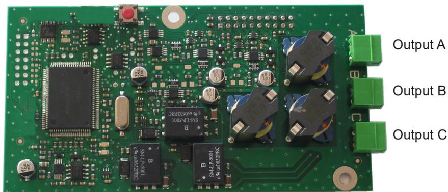
This option board does not require any software programming (by default the time is the local time defined in the Sigma and the line is stopped). Only the time zone differential and the state of the line (On / Off) is to be defined in the “Time outputs” technician menu (see page 35).
