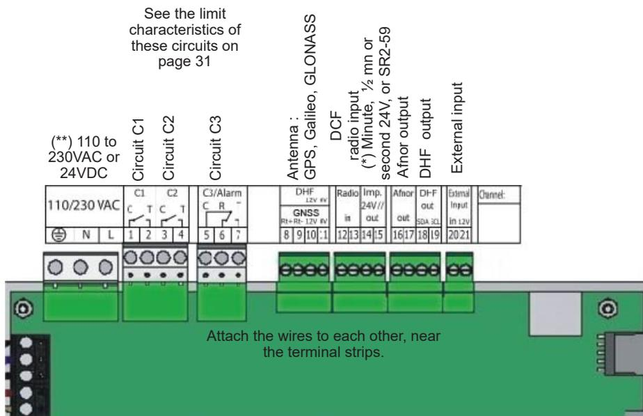
(\* ) See page 25, the “Time outputs” menu to set this output (Pulse minute, ½ minute, second 24V or power TBT 24VDC 0.5A).
