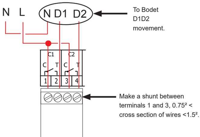
⚠ Circuits must be protected by fuse disconnecter or circuit breaker 4A maximum. Indicate on the label above the terminal block the location of these protections.
