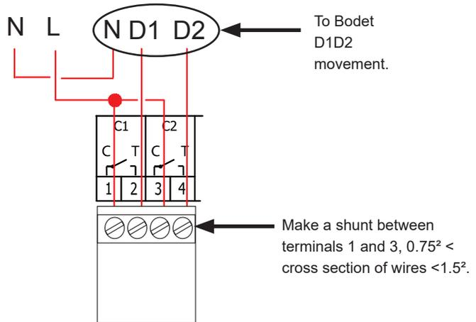
D1 D2 uses the relays of circuits 1 and 2
