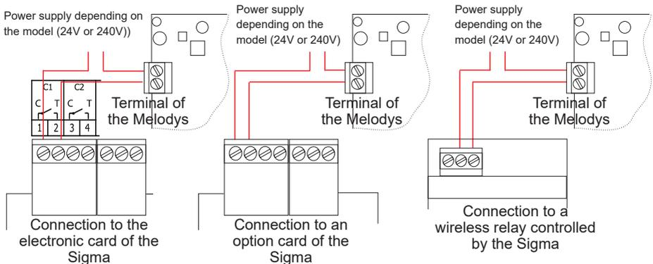
The MelodyS can be connected directly to a relay output of the Sigma, an option card or a wireless relay.
