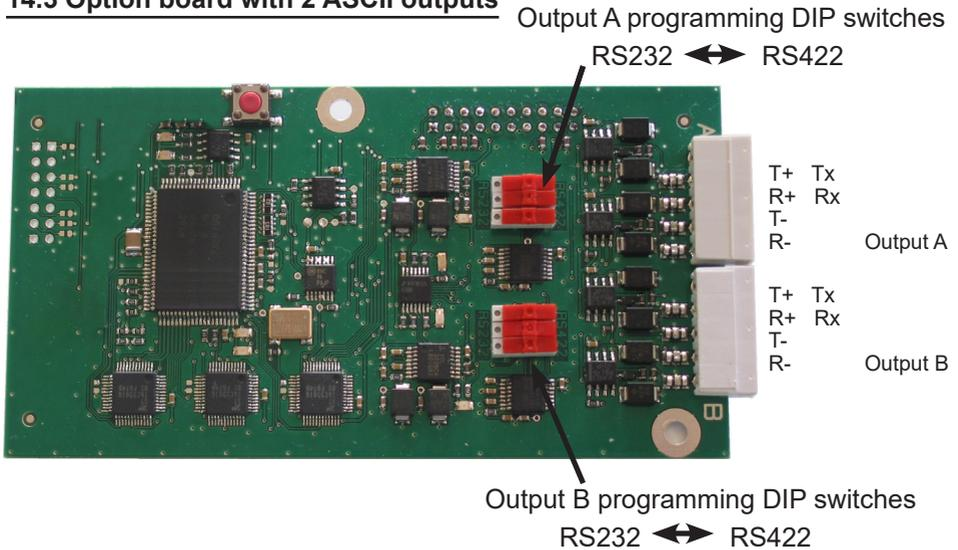
This option board has 2 ASCII outputs which can be configured in RS232 or RS422 (RS485) mode. To change the configuration, push the 3 DIP switches to the desired position.
