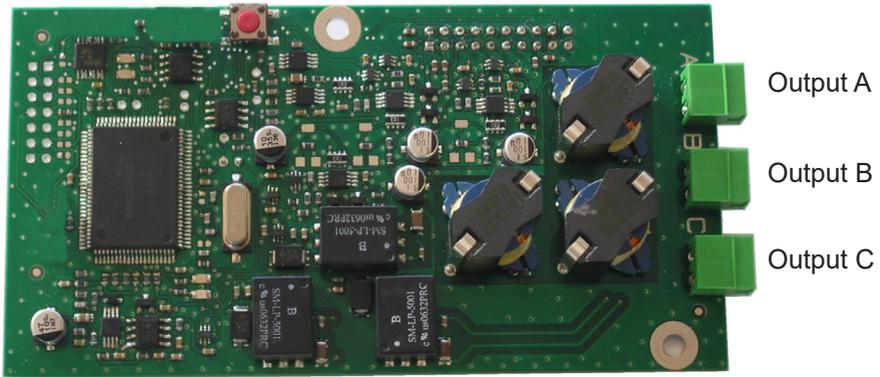
This option board does not require any software programming (by default the time is the local time defined in the Sigma and the line is stopped). Only the time zone differential and the state of the line (On / Off) is to be defined in the “Time outputs” technician menu (see page 36).
