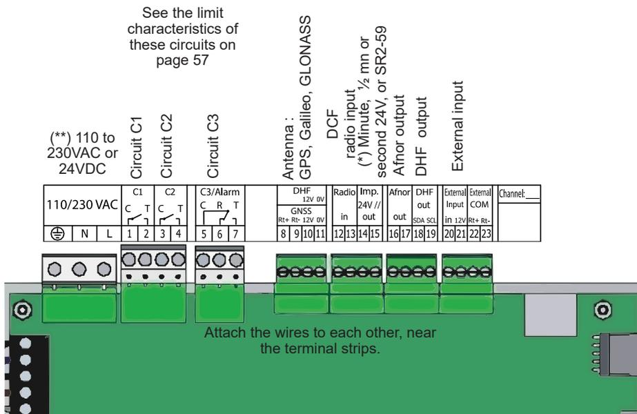
(\*) See page 33, the “Time outputs” menu to set this output (Pulse minute, ½ minute, second 24V or power TBT 24VDC 1A).
