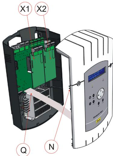
**RACK version :** Open the rack unit and install the option board(s) in the slots provided (X1) to (X2).
