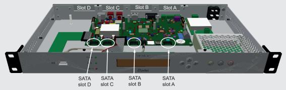
This operation applies to both Network option cards (RJ45 port) and Fibre Network option cards (SFP port). Make sure to connect the SATA cable to the right connector on the motherboard corresponding to the slot where the option card is installed.
