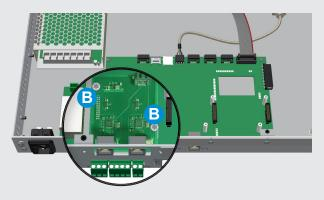
7) Fix the aluminium plate in order to close the space around the option card:
