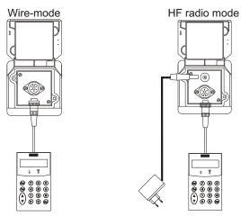
Locking ring of the unit plug must be correctly engaged in order to avoid communication problems.
