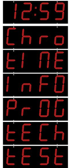
3. Press [S] to validate the choice of menu. Otherwise, press [M] to exit from the programming menu (or press [Sel] button for 3 seconds).
