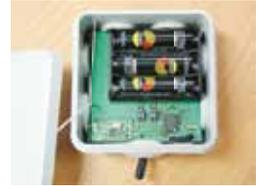
It is recommended to test the HF link before attaching the temperature sensor. Position the plug and the stud before engaging it in the casing. The sensor must imperatively be pointing downwards for obvious waterproofing reasons.
