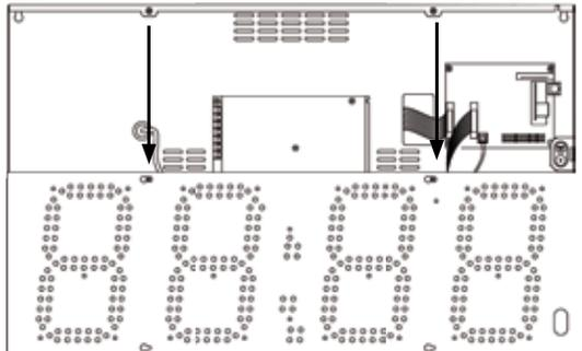
*Tip to open the box : release the screws of the facade and put it on the 2 screws at the bottom*
