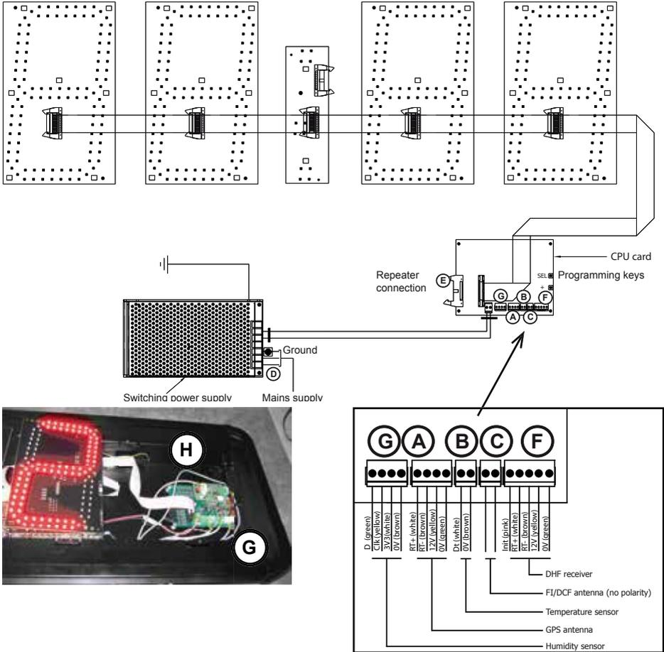
All the cables must be held flat against the casing: use a cable tie at the bottom of the spacers or another system.
