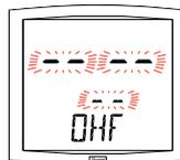
*INIT* : this mode forces the clock to search a DHF transmitter. After selecting this mode, the clock comes back to the time display, initialised to 00h00 01/01/2000. As soon as the clock finds a DHF transmitter, the clock is synchronised and switched to “nor” mode. The clock is now associated and synchronised by this transmitter.
