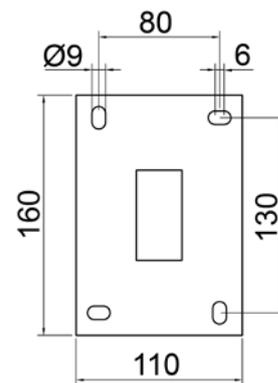
Abmessungen in mm
