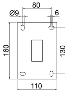
Abmessungen in mm
