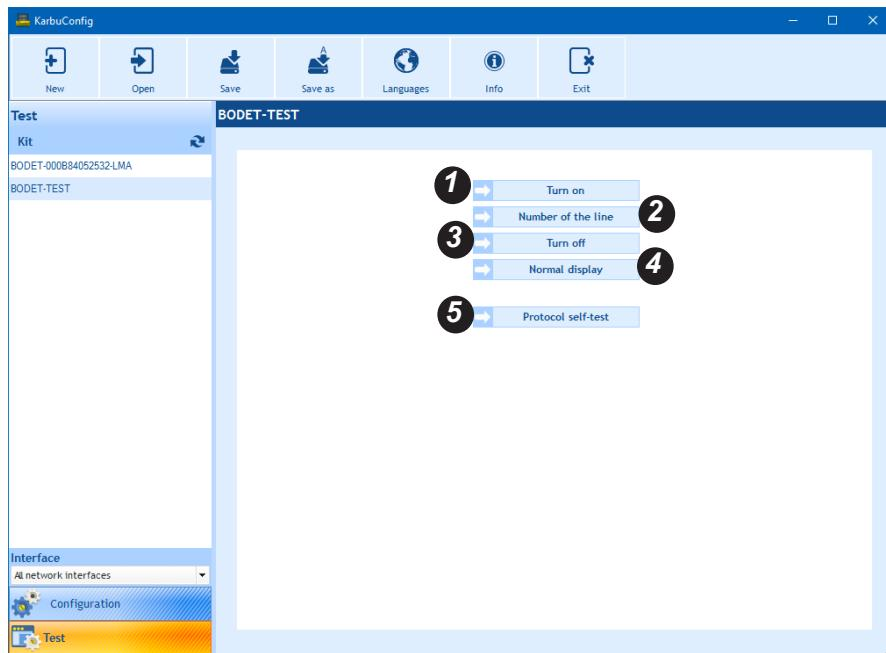
**1** to switch on all the LEDs of each module of lines.
